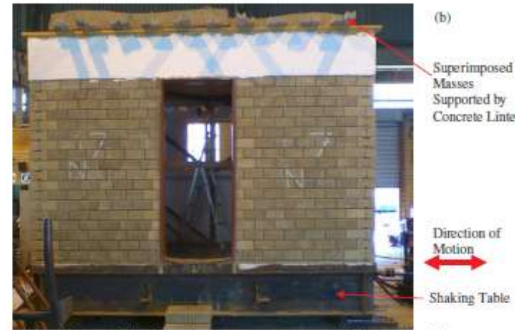
(a) General layout of the dry stack masonry test structure; (b) Photograph of the test structure—North Wall
