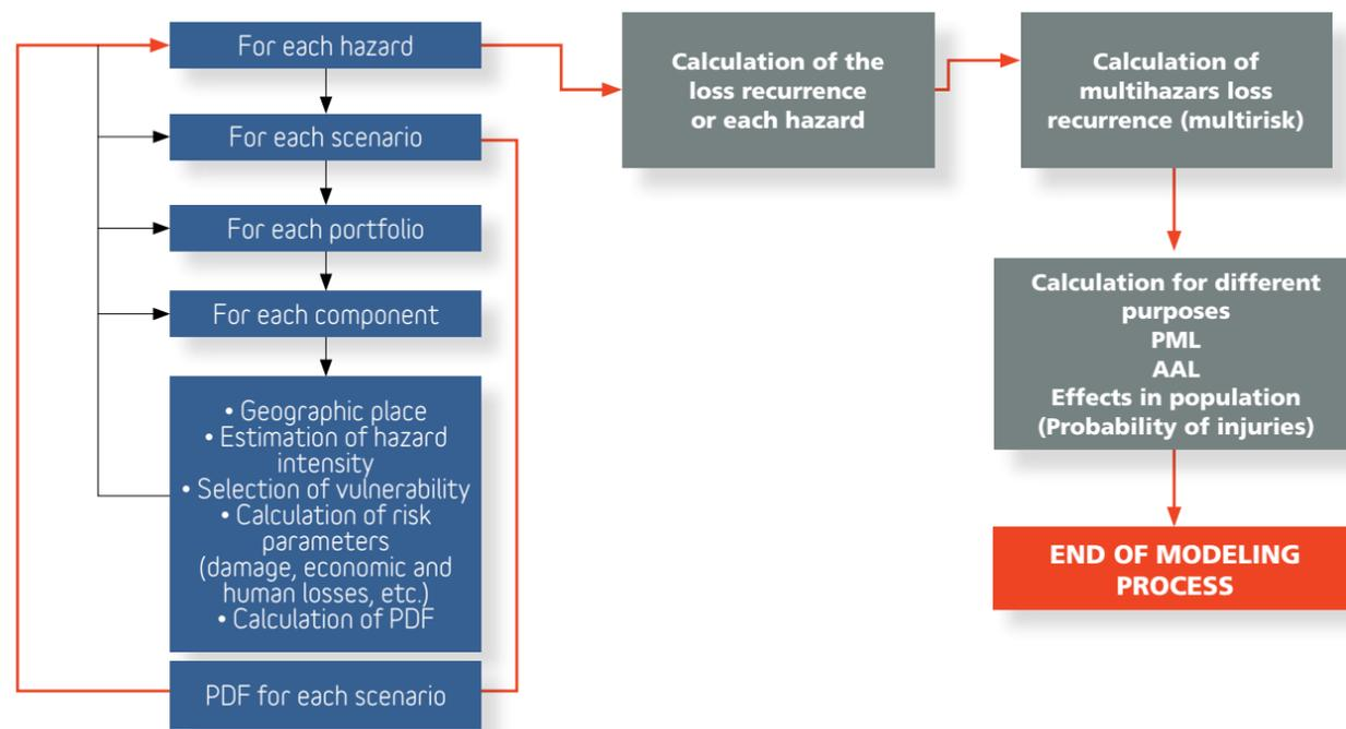
and to identify the buildings and blocks with potential damage concentration. CAPRA is designed to produce, upon the user's request, probabilistic loss results for specific scenarios (Figure 4).
