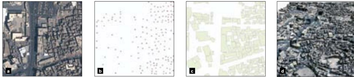
**Figure 2:** The figure shows a 250 x 250 m large area collected over Sana'a and the derived exposure products (a), point assessments (b), building footprint map (c) and building volume map (d)
